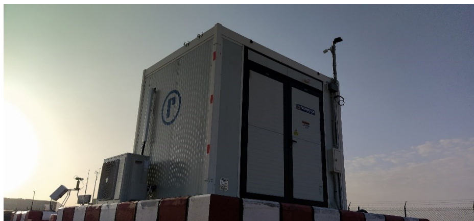
Εικόνα 1: Dust Detection Lidar from Installation at Riyadh Airport
